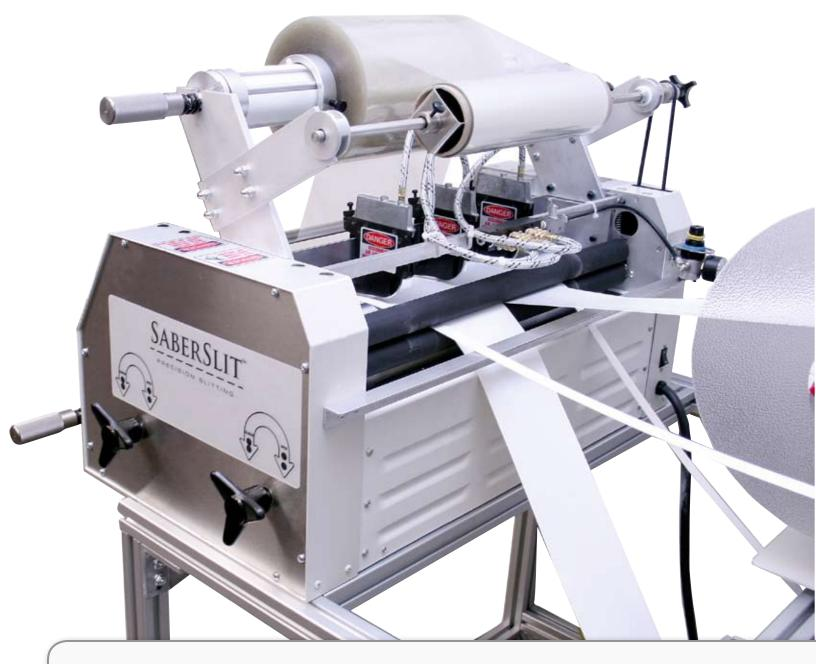
This is the back of the SaberSlit pictured as it laminates and then slits two 6" good rolls and two 1.5" scrap rolls off the edges. Rewinders are collecting both the good material and the scrap material.
