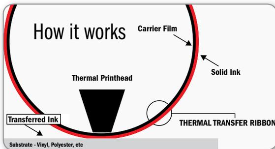
The Edge FX thermal transfer printer uses heat and pressure to transfer resin-based inks. The ribbon and material travel at the same speed so that the printhead applies a continuous image.
